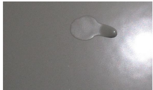
Figure 15 – Paint Drip Surface
