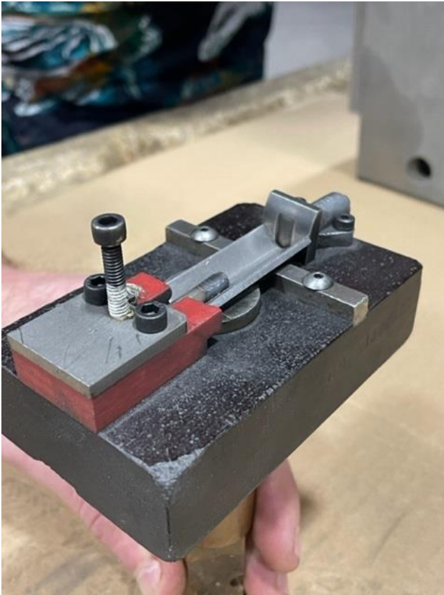
Figure 25 – Adjustable Hinge Pin Alignment Fixture (Perspective View)
