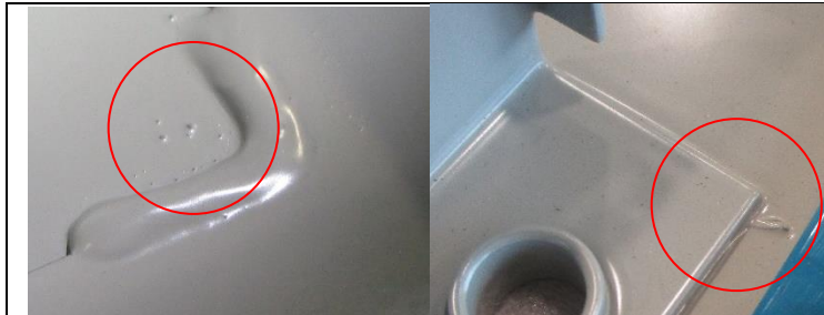
Figure 4 – Random (4 or 5) debris less than 1/8” will be accepted. If debris patterns become greater than 5 or extends to more than 2 surfaces, the process will be deemed out of control and will be unacceptable.
