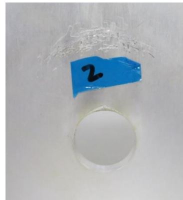
Figure 32 – Damage from Improper Hanging
