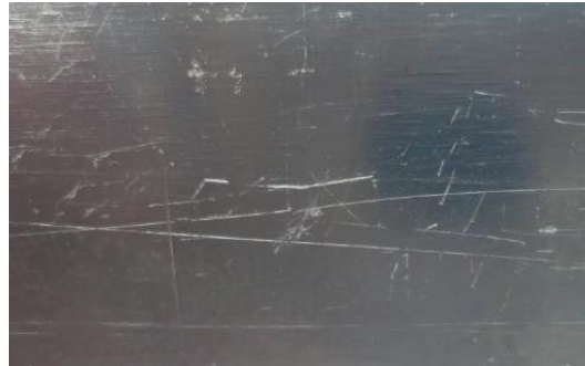
Figure 36 – Scratched Plating (No Copper Exposed)
