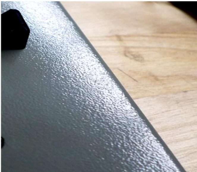
Figure 20 – “Orange Peel” Surface
