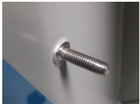
Figure 17 – Damage to Threads That Prevents Hardware Mating
