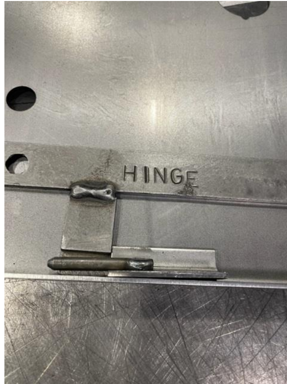
Figure 26 – Pin Assembly Location Fixture
