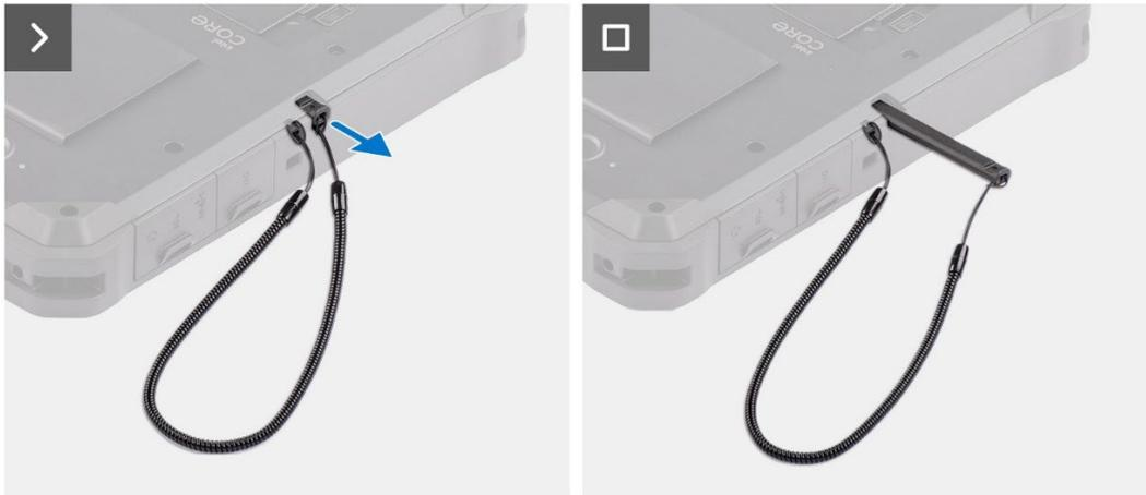
**Figure 54. Replace Stylus and Tether.**
